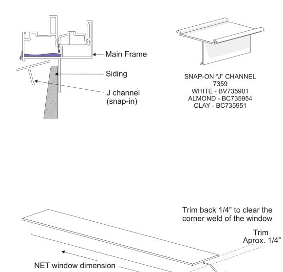
Use silicone sealant to secure the J channel to the frame and at miters
