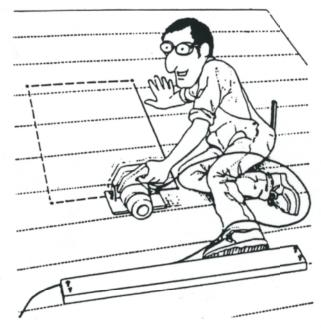
2 Cutting Through. Cut hole in roof to exact inside curb dimension listed for your skylite. Provision has been made for skylite contraction and expansion, but hole must be cut according to instructions to assume proper fit. Check local building codes before cutting any structural members.
