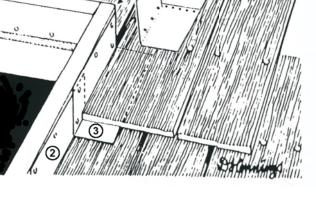
**5** Flashing the curb. Install flashing as illustrated, up the curb to make a neat tight fit. Tack flashing to curb as necessary. One piece head & tail wrap around and seals corners of curb. Underlay shingles with flashing as roofing is built up along the sides of the curb. See steps 1-4 above.
