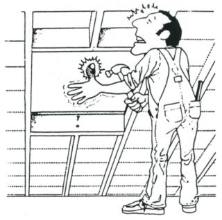
**B** Framing the opening. Check rafter or trusses for dimensions of lumber. Using lumber of the same dimension, frame under deck across opening, to connect rafters or trusses. Form square or rectangle to exact dimensions of opening.
