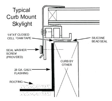
6 Seating skylite on the curb. Apply a continuous strip of 1" wide closed cell foam tape around the outside top of the curb. Place the skylight on the curb and seat firmly in place. DO NOT FORCE SKYLITE. It must fit easily over the curb and flashing. Skylites are secured with a seal washer screw(provided).
