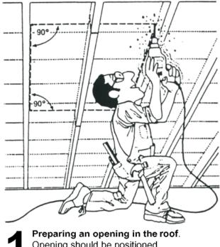
Opening should be positioned between rafters or trusses in accordance with desired day lighting effect. Drill holes through roof from inside at precise corners of the planned skylight opening, using INSIDE curb dimensions.
