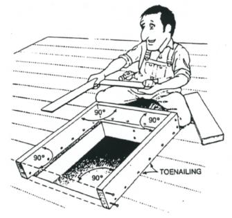
Building the curb. Using 2" x 4" to 2" x 12" lumber build a rectangular frame - or curb mounted flush with the opening. All corners must be 90 degrees. Check to see if your skylite fits the curb. The top of the curb must be flush with the underside of the skylite. Remove unit and proceed to the next step.
